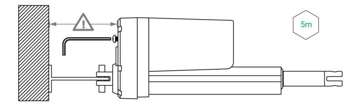
The torque required to manually move the extension tube is within 1.7 Nm, maximum 65 RPM. Please do not run the outer tube to the end of stroke, as that may damage the actuator.
